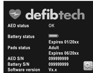
**With the AED off**, press and release the CENTER softkey button (as indicated by the arrow above). Ensure that the AED Status screen appears as shown above and that the “AED Status” is “OK”.
