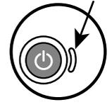
**When the AED is off**, the Active Status Indicator (ASI) should flash green. If the ASI flashes red, is solid red, or if there is no flashing light, the unit requires service.
