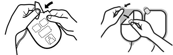
Tear open pads package. → Peel adhesive pads from blue liner.
