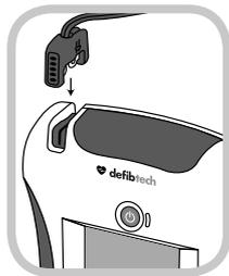
Insert the connector end of the defibrillation pad cable into the pads connector socket on the top-left corner of the DDU-2200 AED as shown. Insert pads connector firmly until it is fully seated in the unit. The connector will only fit in one way – if the connector does not fit, rotate the connector before trying again.
