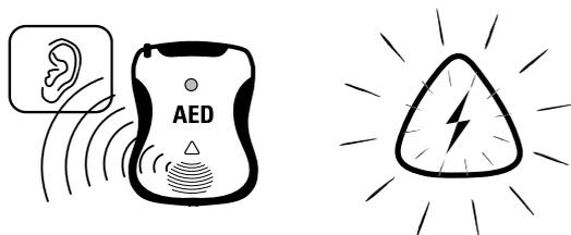
If the DDU-2200 AED determines that a shock is required, the unit will indicate this by a vocal announcement and by flashing the Shock Required Indicator for 5 seconds.
