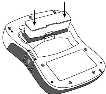
Ensure that the battery pack has not expired. Expired battery packs must not be used. When the battery pack is installed, the AED will turn on and run a battery pack test. Wait for the test to complete and for the unit to turn off. For more information, refer to page 15.
