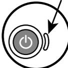
When the AED is off, the Active Status Indicator (ASI) should flash green. If the ASI flashes red, is solid red, or if there is no flashing light, the unit requires service.
