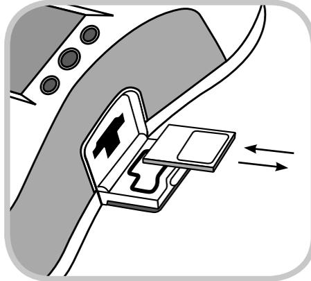
To remove the DDC card, press the card as far as it will go and then release. Upon release, the DDC card will be partially ejected and can be removed by pulling the DDC card the rest of the way out.
